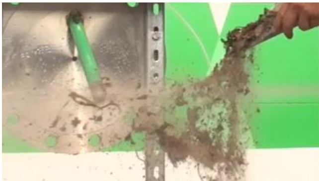
FIGURE 12. HIGH VELOCITY AND WET PROCESS STREAM SIMULATION TOGETHER WITH SAND PARTICLES.
