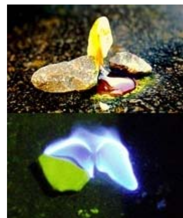
Figure 3: Sulphur melts to a blood-red liquid. When burned, it emits a blue flame and forms SO 2 from: S + O_2 \rightarrow SO_2
