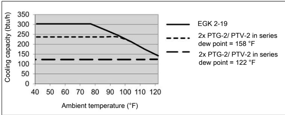
Remark: The limit curves for the heat exchanger apply to a dew point of 158 °F under standard conditions per DIN EN 15267-3:2008-03 and to a dew point of 122 °F under operating conditions.
