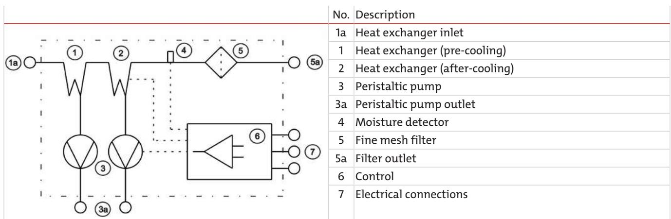
The gas to be conditioned is fed directly into the inlet of the heat exchanger (1, 1a). A hose is pre-installed between the heat exchanger (2) outlet and the fine mesh filter (5). Sample gas is continued directly from the outlet of this filter via hose fitting (5a).
