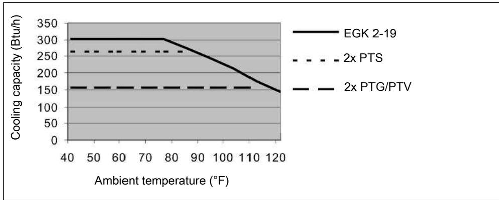
Note: The limit curves for the heat exchangers exchanger apply to a dew point of 104 °F.
