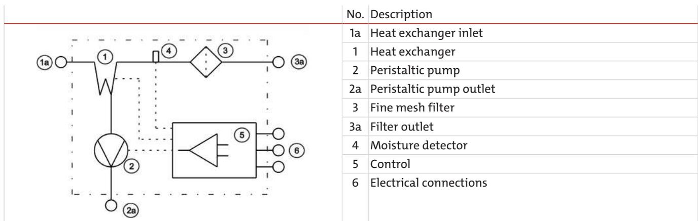
The gas to be conditioned is fed directly into the inlet of the heat exchanger (1, 1a). A hose is pre-installed between the heat exchanger outlet and the fine mesh filter (3). Sample gas is continued directly from the outlet of this filter via hose fitting (3a).
