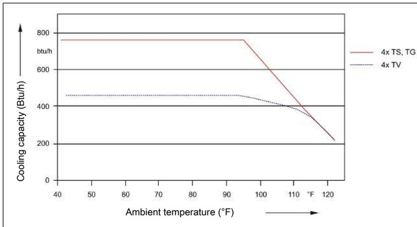
Note: The limit curves for the heat exchangers exchanger apply to a dew point of 149 °F.
