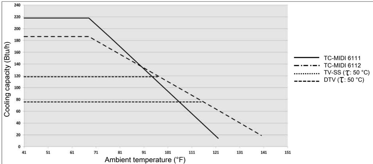
Note: The limit curves for the heat exchangers exchanger apply to a dew point of 122 °F.
