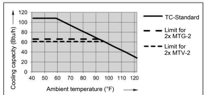
Note: The limit curves for the heat exchangers MTV-2 and MTG-2 apply to a dew point of 122 °F.
