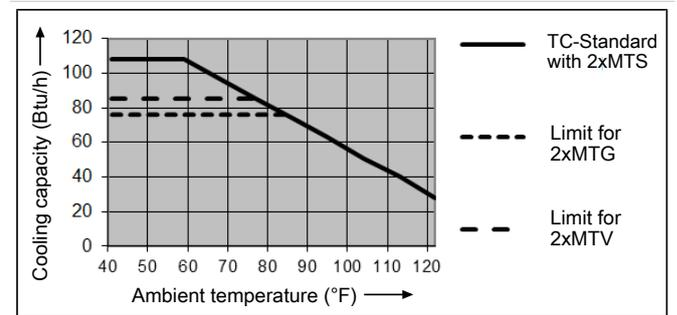
Note: The limit curves for the heat exchangers exchanger PTG, PTV or MTV apply to a dew point of 104 °F.
